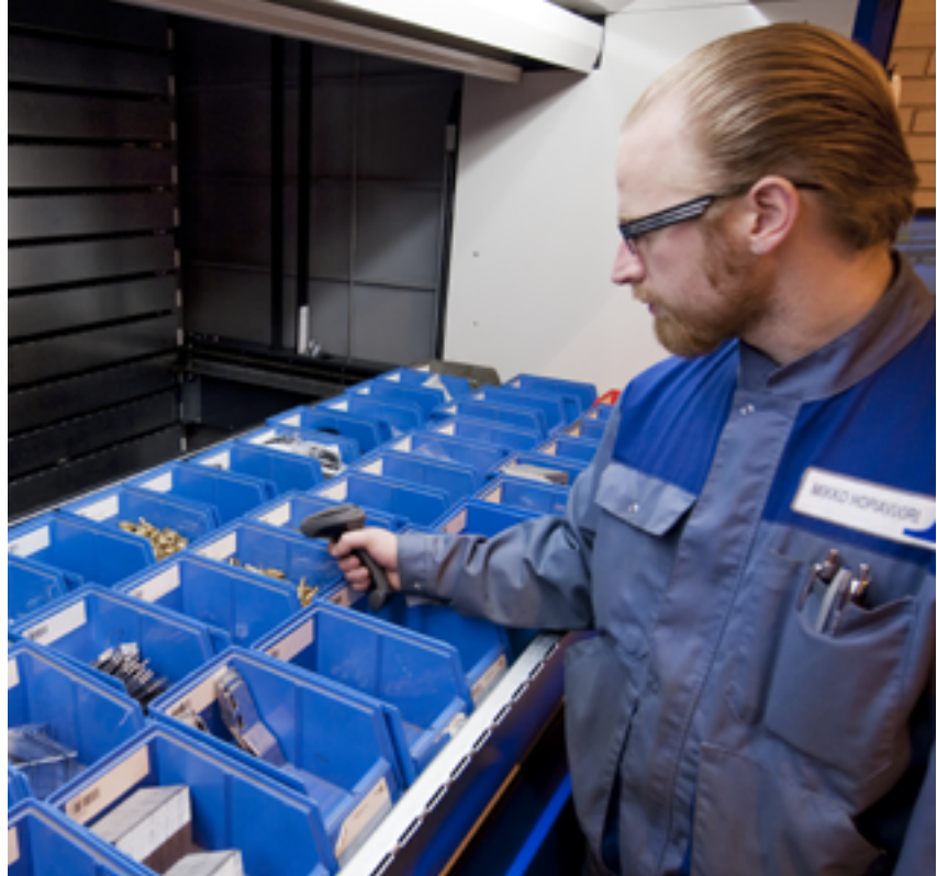
Automated storage machines can be combined with wireless barcode reader and pack to light systems for fast batch processing.
